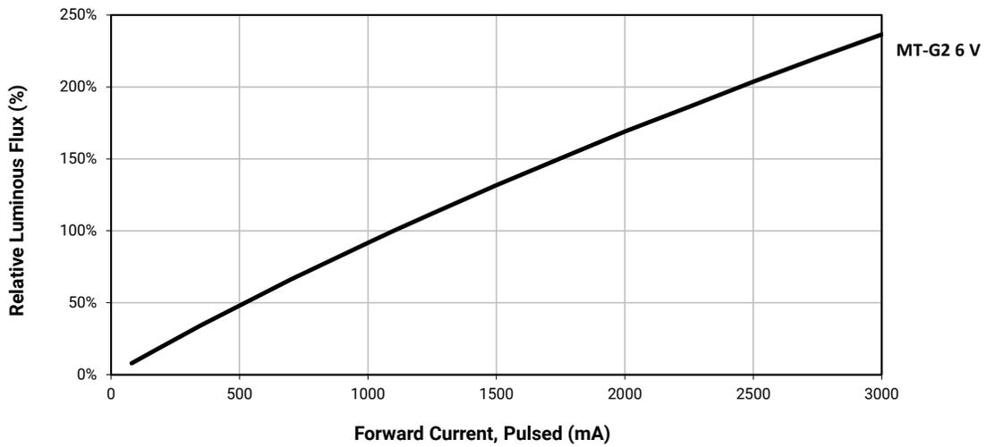
RELATIVE LUMINOUS FLUX VS. CURRENT ( $T_j = 85\text{ }^\circ\text{C}$ ) - CONTINUED
