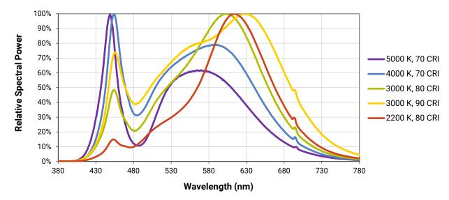
The following graph is the result of a series of pulsed measurements at 550 mA and  $T_J$  = 85 °C.
