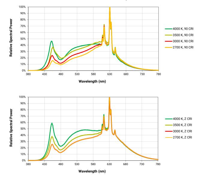
The following graphs are the result of a series of pulsed measurements at 450 mA and T<sub>1</sub> = 85 °C.
