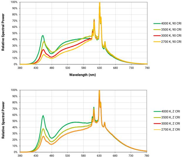
The following graphs are the result of a series of pulsed measurements at 1080 mA and T<sub>1</sub> = 85 °C.
