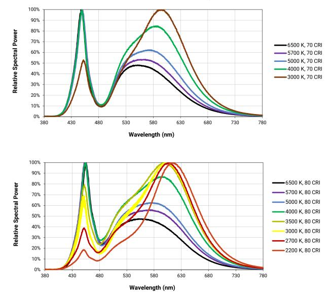
The following graphs are the result of a series of pulsed measurements at 540 mA and  $T_{J}$  = 85 °C.
