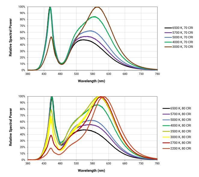
The following graphs are the result of a series of pulsed measurements at 180 mA and  $T_{J}$  = 85 °C.
