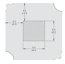
Tc measurement point: either the anode or cathode solder pad
