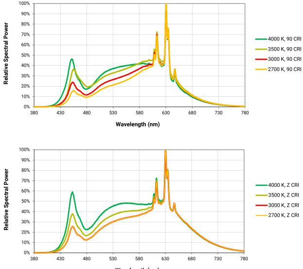
The following graphs are the result of a series of pulsed measurements at 90 mA and T<sub>1</sub> = 85 °C.
