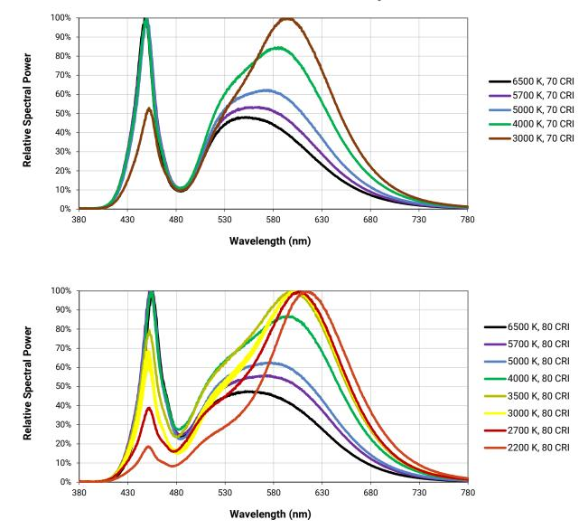
The following graphs are the result of a series of pulsed measurements at 1300 mA and T<sub>1</sub> = 85 °C.
