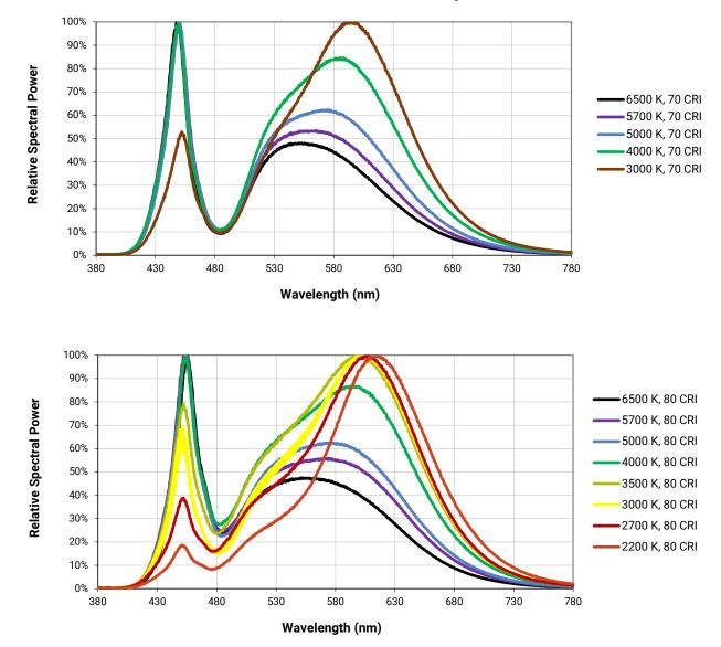
The following graphs are the result of a series of pulsed measurements at 700 mA and T<sub>1</sub> = 85 °C.
