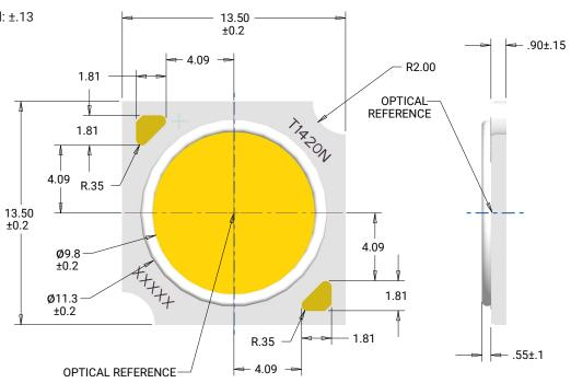
Tc measurement point: either the anode or cathode solder pad
