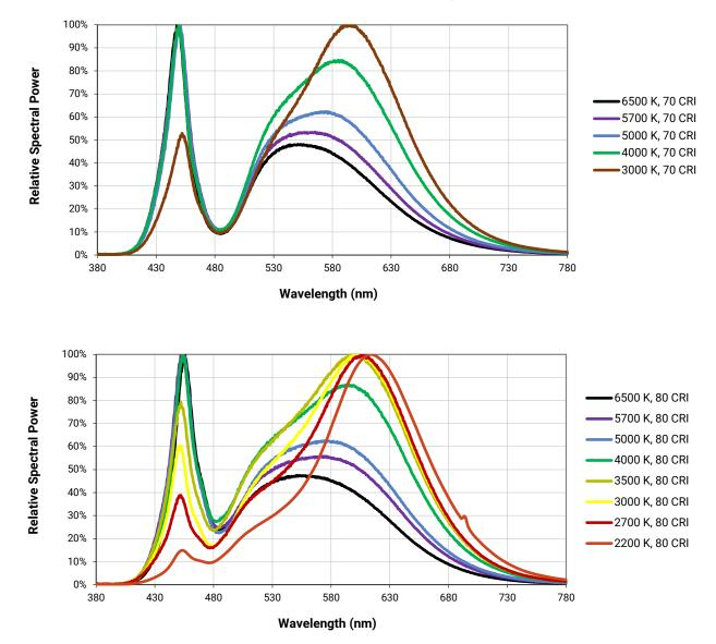
The following graphs are the result of a series of pulsed measurements at 200 mA and  $T_{J}$  = 85 °C.
