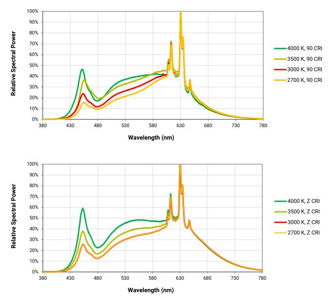
The following graphs are the result of a series of pulsed measurements at 700 mA and  $T_{J}$  = 85 °C.
