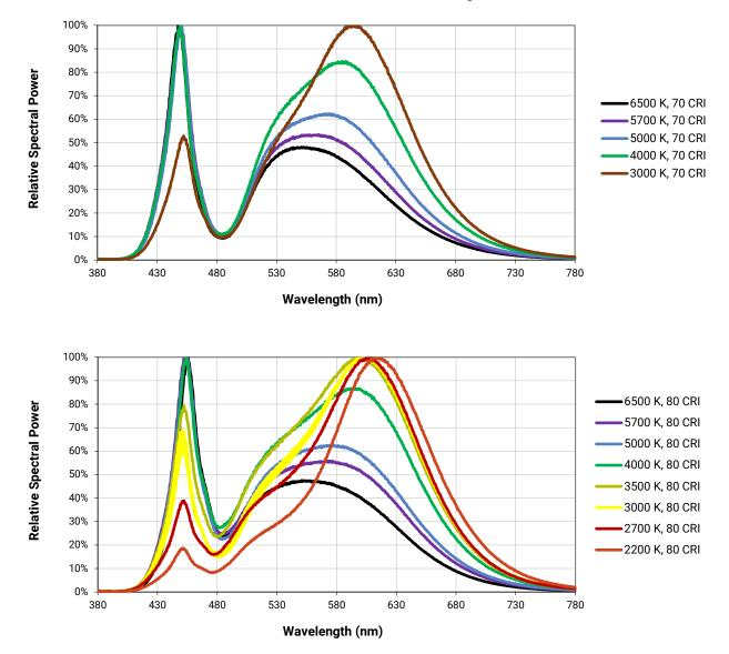
The following graphs are the result of a series of pulsed measurements at 500 mA and T<sub>1</sub> = 85 °C.
