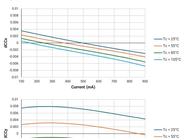
• Relative Chromaticity versus Current and Temperature are shown for reference only. These graphs are not a specification.
