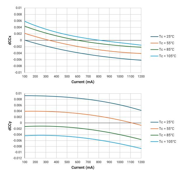
• Relative Chromaticity versus Current and Temperature are shown for reference only. These graphs are not a specification.
