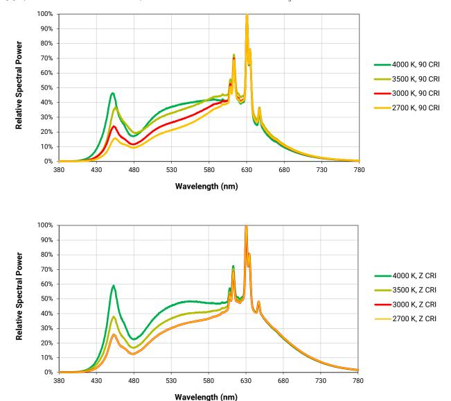
The following graphs are the result of a series of pulsed measurements at 1100 mA and  $T_1 = 85$  °C.
