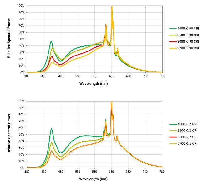
The following graphs are the result of a series of pulsed measurements at 450 mA and  $T_J$  = 85 °C.
