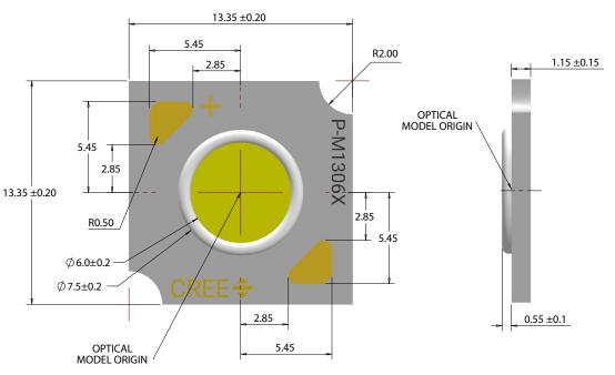
Tc measurement point: either the anode or cathode solder pad
