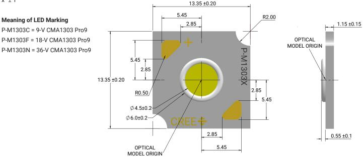
Tc measurement point: either the anode or cathode solder pad
