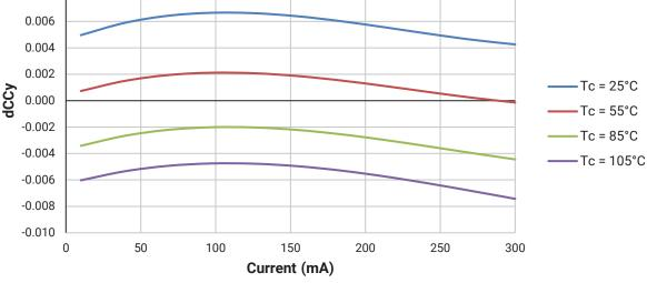
· Relative Chromaticity versus Current and Temperature are shown for reference only. These graphs are not a specification.
