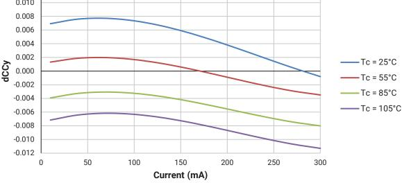
• Relative Chromaticity versus Current and Temperature are shown for reference only. These graphs are not a specification.
