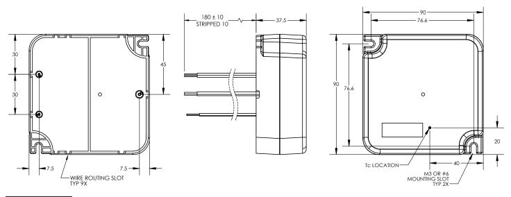
Dimensions for all the diagrams are in mm and are for reference only. For exact dimensions and tolerances, refer to the 3-D models (.STEP files) for the LMD300, LMD400 and LMD600 drivers available by selecting the Documentation tab on the LMH2 product page.
