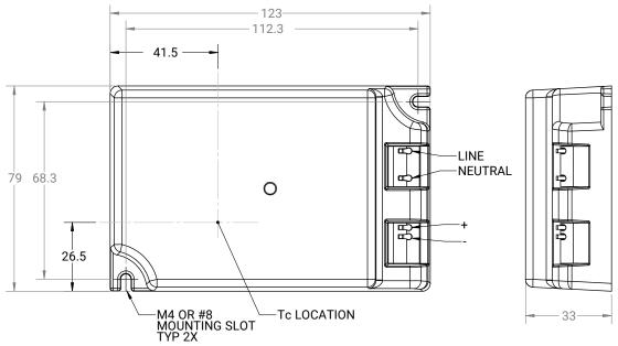
Dimensions for all the LMD125 diagrams are in mm and are for reference only. For exact dimensions and tolerances, refer to the 3-D models (.STEP files) for the LMD125 drivers available by selecting the Documentation tab on the LMH2 product page.
