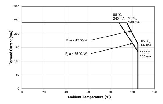
The maximum forward current is determined by the thermal resistance between the LED junction and ambient.
