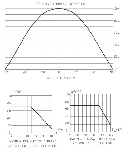
The graph shows the maximum allowable DC current for a LED die of each color.
