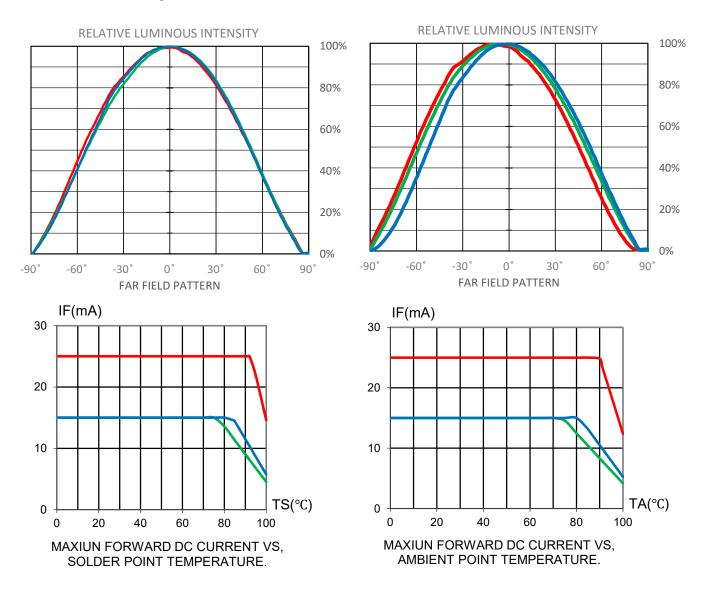
The graph shows the maximum allowable DC current for a LED die of each color.
