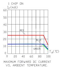
The graph shows the maximum allowable DC current for a LED die of each color.
