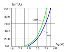
FIG.1 FORWARD CURRENT VS. FORWARD VOLTAGE.
