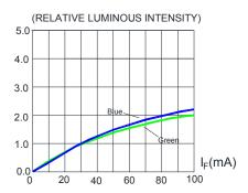
FIG.2 RELATIVE LUMINOUS INTENSITY VS. FORWARD CURRENT
