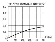
FIG.2 RELATIVE LUMINOUS INTENSITY VS. FORWARD CURRENT
