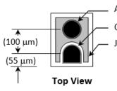
Anode (+), Ø 80 μm, Bond Area, Ø 70 μm
