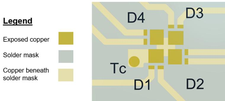
Figure 9: XE-G 200- $\mu$ m spacing PCB design
