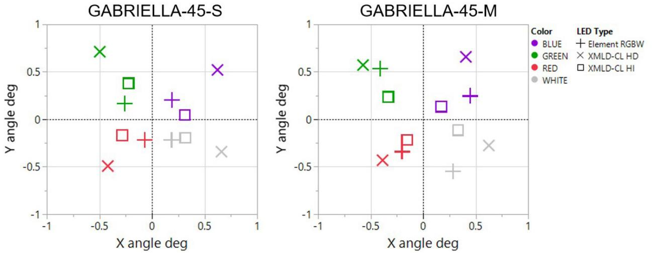
Figure 8: Optical peak intensity displacement of each color diode in an RGBW array, in degrees from center. The XE-G RGBW array at 200- $\mu$ m spacing has similar performance to XM-L Color Gen 2 HI.
