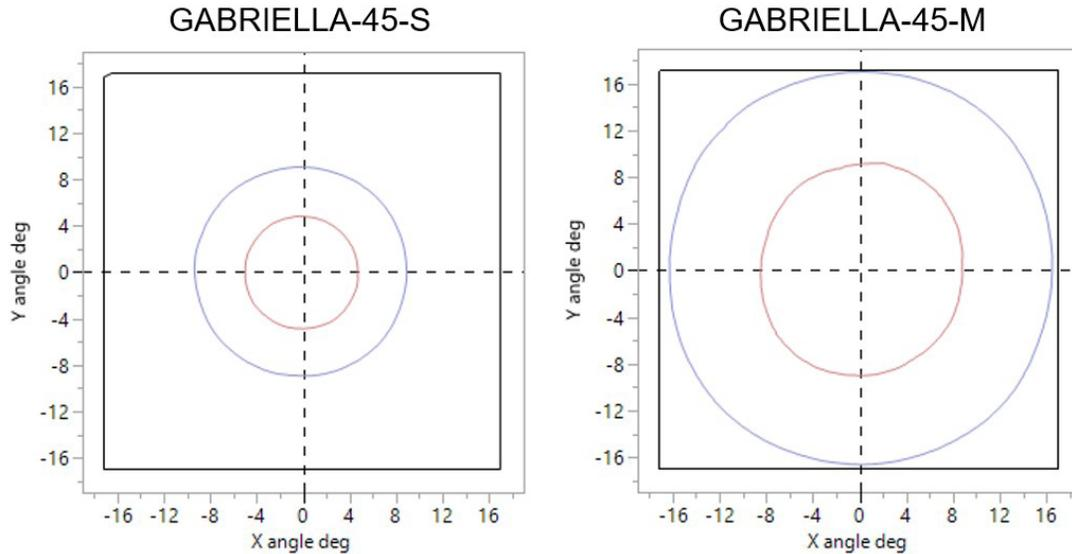
**Figure 5: 50% intensity (light red) and 10% intensity (blue) contour curves for an XE-G RGBW pinwheel array with 200- $\mu$ m spacing in the Gabriella-45-S optic (left) and Gabriella-45-M optic (right) projected onto a flat surface. The Spot optic gives a roughly 9° beam angle and 19° field angle, while the Medium optic gives a roughly 17° beam angle and 32° field angle.**
