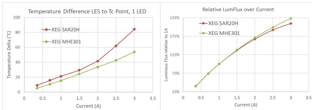
**Figure 13: Difference between LES temperature and T<sub>c</sub> measuring point (left) and luminous flux (right) of individual white XE-G LEDs mounted on starboards with a direct thermal path (MHE<sup>®</sup>301) and without a direct thermal path (SAR20H)<sup>1</sup>.**
