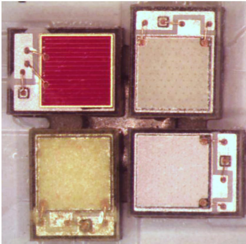
Figure 1: XE-G RGBW array with average gap between LEDs of 200  $\mu\text{m}$
