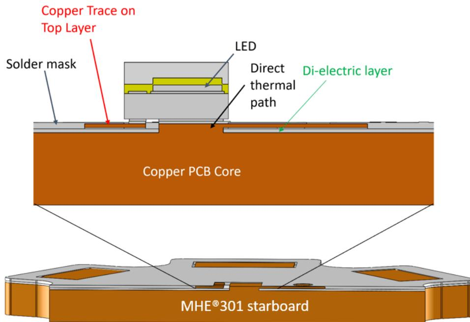
Figure 12: Cross-sectional view of an XE-G LED soldered onto a single-component starboard designed with Rayben's MHE<sup>®</sup> 301 direct thermal path technology. The copper core protrudes upward only in the thermal pad location to make direct contact to the LED for better heat sinking.
