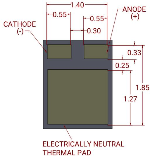
Figure 11: Bottom View of XE-G LED
