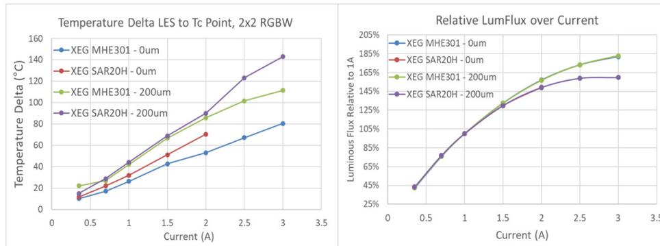
**Figure 14: Difference between LES temperature and Tc measuring point (left) and luminous flux (right) of a RGBW Pinwheel array of XE-G LEDs mounted on 50 mm PCBs with a direct thermal path (MHE<sup>®</sup>301) and without a direct thermal path (SAR20H).**
