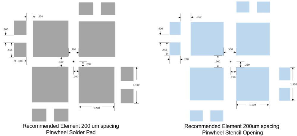
Figure 10: Copper pad layout (left) and stencil dimensions (right) used for a 200- $\mu\text{m}$  spacing in a 2x2 array
