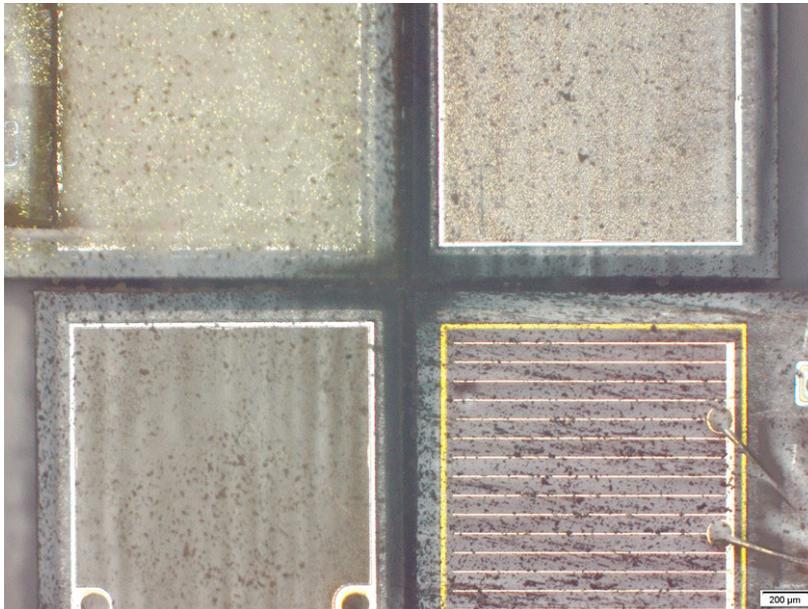
Figure 3: XE-G 4-LED pinwheel array with designed 0- $\mu\text{m}$  spacing. Actual spacing is about 50  $\mu\text{m}$ , as shown by the scale bar in the lower right. This array was created using standard pick and place equipment normally capable of a minimum 200- $\mu\text{m}$  spacing.
