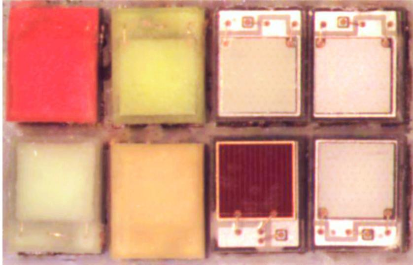
Figure 2: A 4x2 array of XE-G LEDs with average spacing of 200  $\mu\text{m}$ . Note that the blue and cyan LEDs (right side) are kept far from the LEDs with heavy phosphor coverage to reduce unintended phosphor excitation and improve blue saturation.
