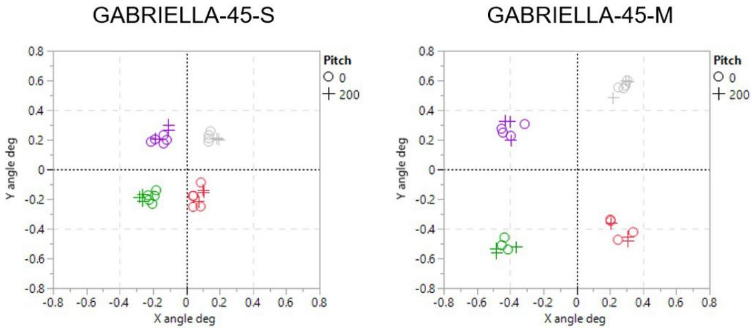
**Figure 4: Location of peak intensity of each color in the array, shown as displacement from center in degrees. The Spot optic had an average of 0.2° displacement per color and the Medium optic had an average of 0.4° displacement per color. Very little difference was observed between 200- $\mu\text{m}$  spacing and the “0- $\mu\text{m}$ ” spacing.**
