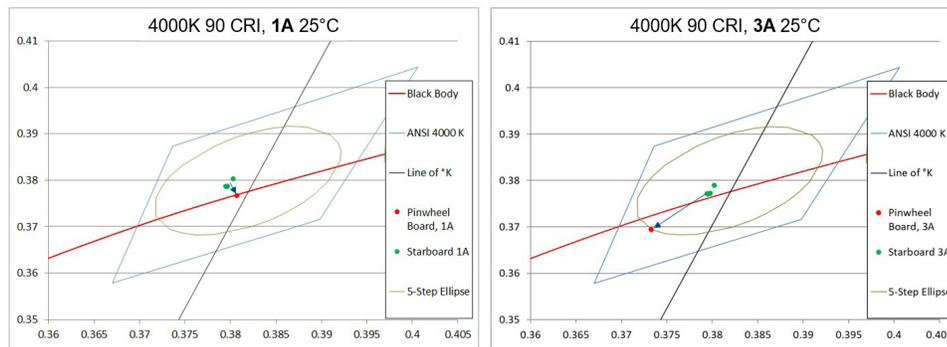
Figure 7: Color shift of close-packed 2X2 array (50- $\mu\text{m}$  pitch)
