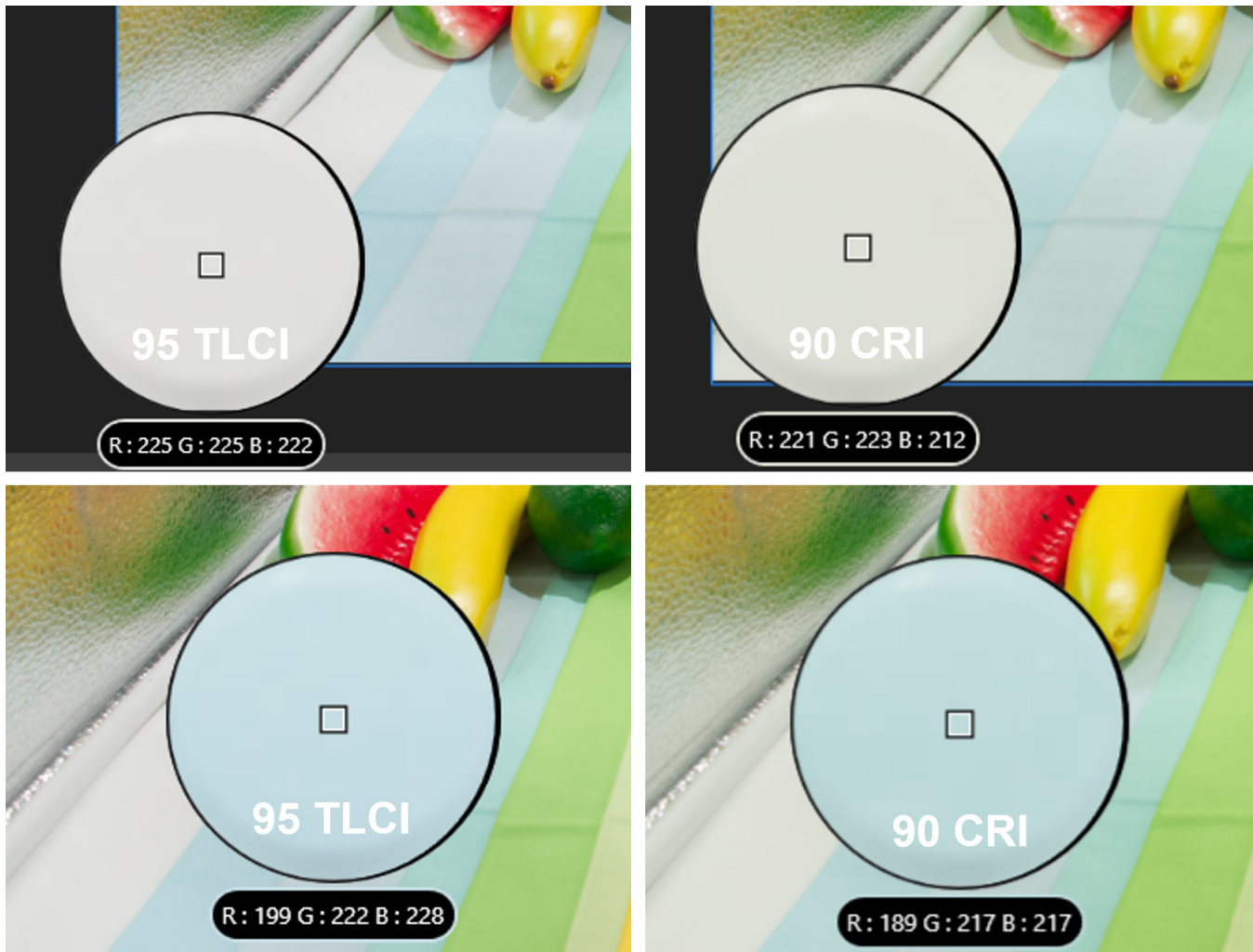
Figure 8: Comparison of digital RGB values on white (top) and cyan (bottom) fabric swatches. TLCI and CRI values of the illumination are inset in the zoom circles.
