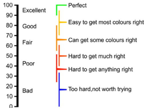
Figure 2: The effort and skill needed (right) to properly color correct photography or videography illuminated by lights of a typical TLCI value of the scale on the left. [2]
