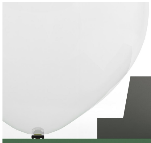
Figure 6: Light not blocked by components near the LED
