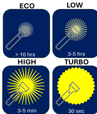
Figure 1: Graphical representation of a flashlight with four output modes along with relative runtimes for each mode.
