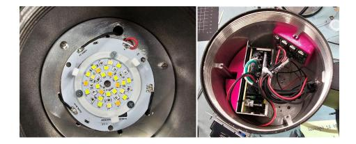
The downlight was assembled into a demonstration to show color mixing, controlled by two linear potentiometers that allow users to adjust the CCT and brightness. The demo was able to be tuned to adjust across a wide range of CCTs while maintaining consistent brightness and high CRI.
