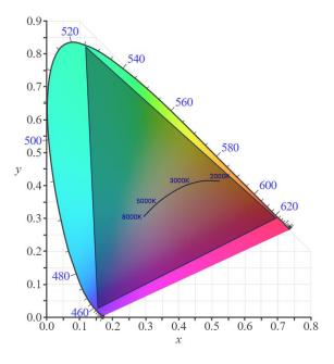
This arrangement might be chosen in an application where the goals are to maximize the available color space for entertainment lighting while minimizing the cost and channel count. Rendering white light with high CRI is not required. Efficacy is not a criterion.
