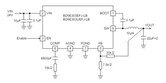
The IC regulates the output by maintaining the feedback pin (FB) at 1.0 V, and this voltage is set up to be ratiometric to the output voltage via a voltage divider. To convert this design to constant current, a signal needs to be created that is ratiometric to the LED current, and that outputs 1.0 V at the 2.0 A-current setpoint. This can be accomplished with an op amp set up in a non-inverting amplifier circuit and using a current-sensing resistor to measure the LED current.
