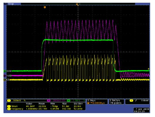
Since the design will operate with a larger voltage difference from input to output than the test shown, and because there is plenty of room to slow down the switching frequency, a larger inductance is chosen. It will be easier to source components with common values, so values of 4.7  $\mu$ H or 10  $\mu$ H are good choices to raise the value. The predicted switching frequency can be calculated from the equations in the data sheet.
