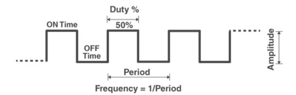
Generally, a microcontroller is needed to generate the PWM signal. Other options including FPGA or ASIC could perform this task as well, but a microcontroller gives more flexibility in this role, particularly during development. This document will focus on microcontroller designs.
