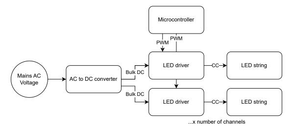
In some applications, a dedicated LED driver IC is available to create a suitable LED driver. In other cases, a constant-current output IC is not available, and the more common constant-voltage type must be adapted to form an LED driver. In either case, some basic criteria are used to select an IC:
