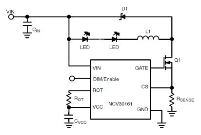
Since the IC's current sense voltage is 200 mV,  $R_{SENSE}$  will be set to 0.1  $\Omega$  to get a 2 A output current (R = V/I = 0.2 V/2 A = 0.1  $\Omega$ ). Other critical components to create the driver include the inductor L1, the freewheel diode D1, and the switching MOSFET Q1.
