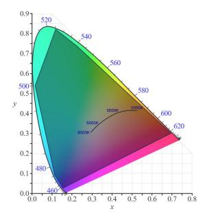
The arrangement of one color point per control channel is not always the case; in advanced color mixing applications a designer might mix multiple LED colors on a single control channel. This is typically done to create a virtual anchor point at a different point in the color space that is not otherwise achievable. It can also be done for CRI or efficacy reasons. This document will only focus on designs with one color point per channel.
