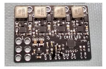
An aluminum-core PCB was designed for four strings of J Series 2835 LEDs and retrofitted into an off-the-shelf sconce downlight. The electronics were powered by a 36 V AC to DC power supply and installed in the back of the downlight.
