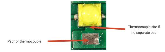
It is not required to use a solder footprint for the thermal pad that is larger than the XLamp XB Family LED itself. In testing, Cree LED has found such a solder pad to have insignificant impact on the resulting T<sub>s</sub> measurement.
