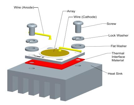
Cree LED recommends the following at all times when handling XLamp CM family LEDs or assemblies containing XLamp CM family LEDs:
