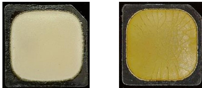
Figure 2: Example images of two devices post the UV exposure test. On the left is the outdoor qualified Cree LED CLY6 part and on the right is an internal control part with no UV protection included.
